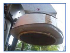
Discharge chute with endless bagger or into a bin.
