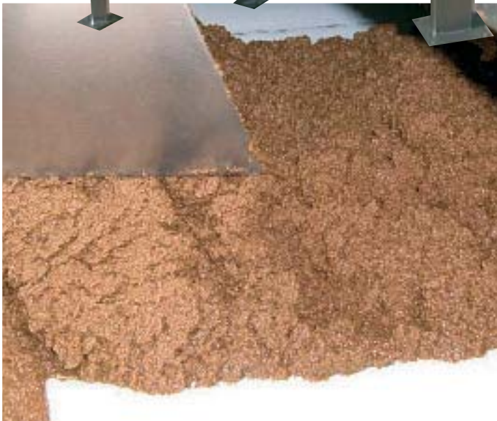
Fango addensato Thickened sludge
